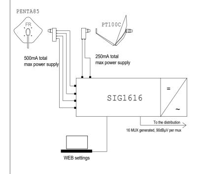
The new SIG1616 compact headend can handle up to 16 different SAT trasponders and remodulate the desired programs on 16 indipendent DVB-C Digital Multiplex, 90dBµV each.
