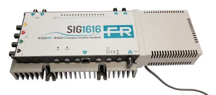
The SIG1616 satellite compact headend is a 16 FTA channels transmodulator with DVB-S/S2 input and 16 DVB-C output muxes. It has 4 main and 2 auxiliary SAT ports for connecting SAT signal.
